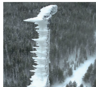
Wind vane on the measurement mast in wpd's Nuolivaara project in Finland: The degree of icing is also monitored on the basis of the camera images
