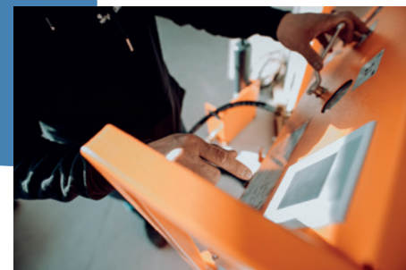
SF6 service unit being used to check the gas level
