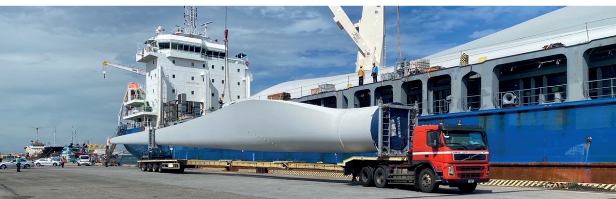
Transporting a rotor blade from quayside into storage after unloading
